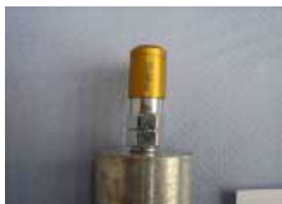
Test sample steel after removing salt residues
