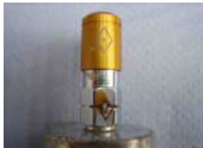
Beginnings of corrosion on steel version
