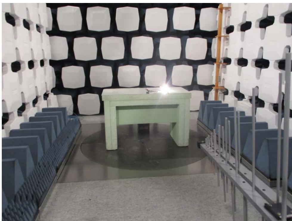
Figure 1: Radiated emission test
